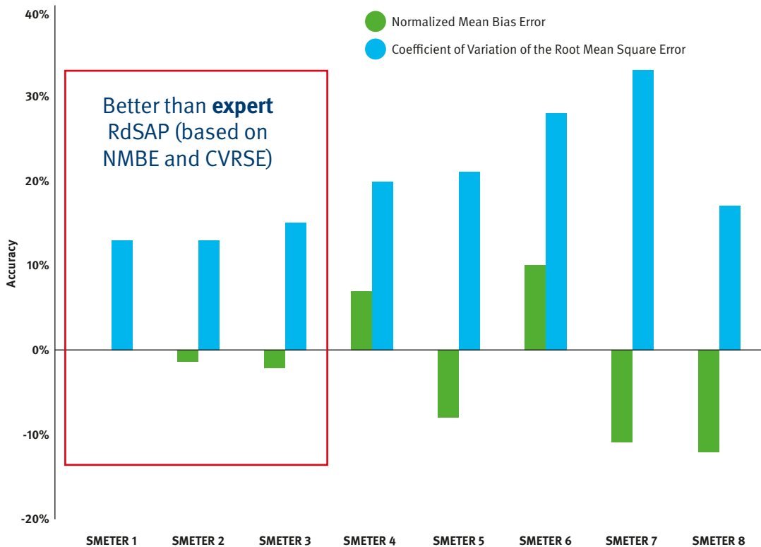
Figure 7: Accuracy (NMBE and CVRMSE) of the in-use HTC generated using SMETERs compared to in-use HTC using modified co-heating test. Three SMETER products were more accurate than the expert RdSAP calculation of HTC.
